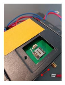
Peel off the double-sided tape on the back of the mobile module (2) and place the rubber sealing washer (12) on the antenna connector. Insert the antenna connector through the designated hole on the side of the Easy-Kirr Control Box (1). Tighten the antenna (4) from the outside, ensuring the rubber sealing washer (12) is on the inside. Press the mobile module (2) firmly against the rear wall of the control box (1).
